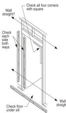
Is the opening the correct size for the door unit? Check it against the door frame size now, before installation. The opening should be frame height plus 1/2 inch, and frame width plus 1/2 inch to 3/4 inch. Fix any problems now.
