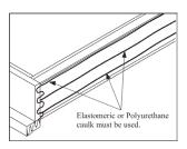
surface of the sill can be caulked. Place very large beads of caulk across the full width of the sill. Additionally, place beads of caulk along the junction of the sill and the jamb and on the bottom surface of the jambs and brickmould.
