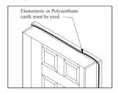
entire perimeter of the door unit. A 1/2 – 5/8 inch bead of Elastomeric or Polyurethane caulk is essential.
