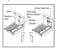
Apply sealant (Polyurethane or Elastomeric) at the joint where the threshold cap meets the door jambs.
