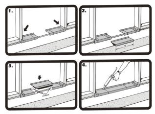
Note: Use only the PVC cement provided in the sill pan kit to glue the pieces together. The sill pan must be sealed to the sub-floor using an Elastomeric or Polyurethane sealant, but do not apply sealant to the bottom of the sill when using a sill pan.
