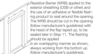
**Use a Sill Pan:** We recommend you first "dry fit" the sill pan in the opening,
