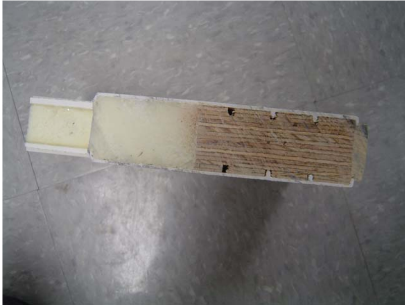
Leaf Cross Section at Lock Stile
